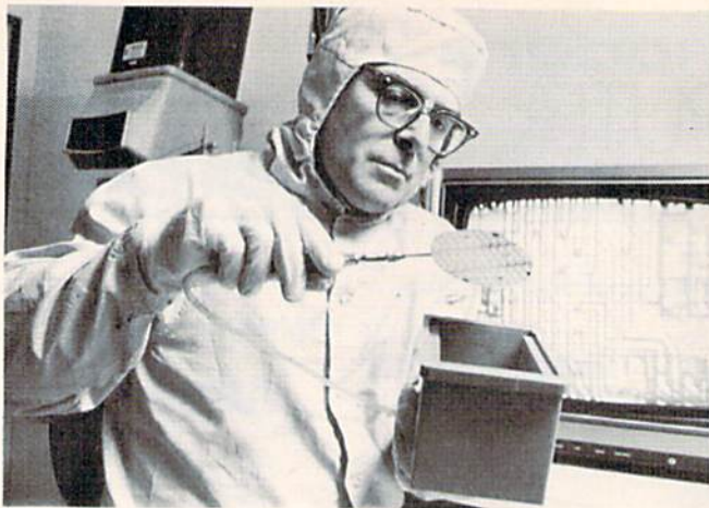
Engineer Mike Grieco at Bell Labs holds a wafer with 64 tiny chips. Behind him you can see a TV picture of the transistors on just one chip magnified 400 times.
